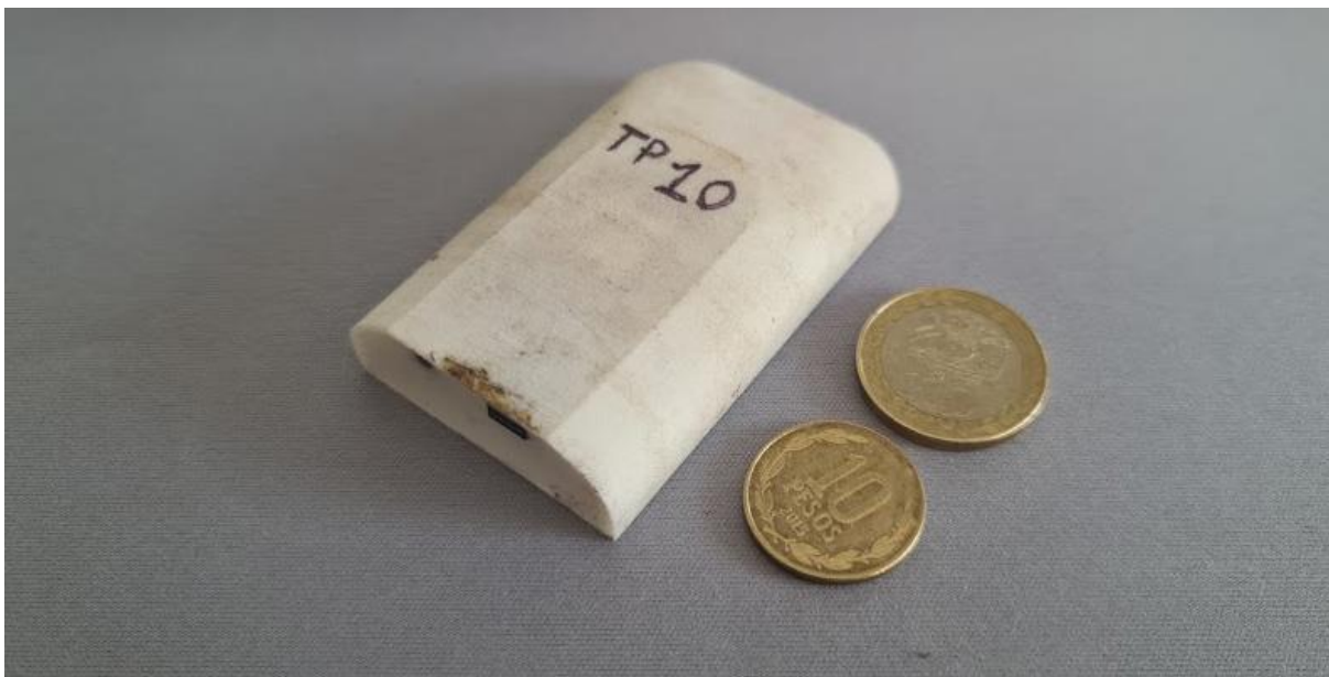
Figure 14 AxyTrek Marine GPS dive logger. 100- and 10-Peso coins for scale.
